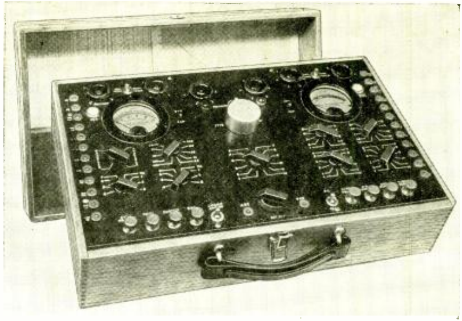
This "laboratory," the new Supreme Master AAA-1 tester, permits "free reference" or point-to-point tests.
