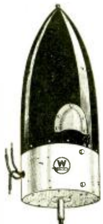
Outside View of Aircraft Generator
